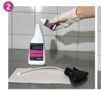
Empty component B completely into component A and blend it well (pivot 3-5 times). The gel should now have a consistant purple colour. Spray some gel into the drain before use, because the gel might have changed colour inside the bottle-tube
